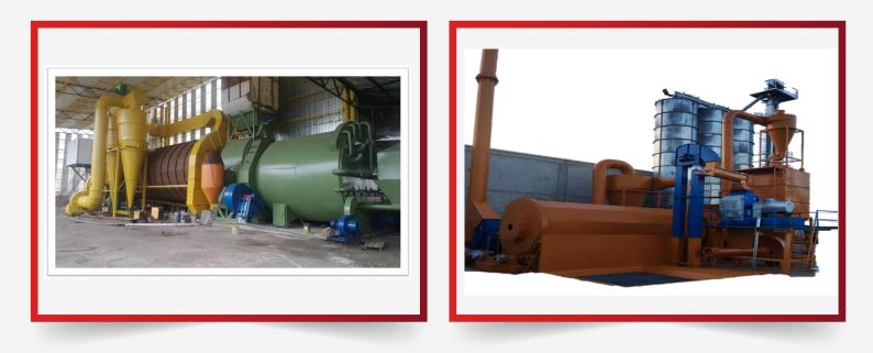
The founders of Enkur Makine are experienced in rotary dryer and stoker cooker. As Enkur Makine, we carry out the drying process of raw materials by drawing the heat we provide in solid fuel furnaces into the rotary dryer. As Enkur Makine, we are able to dry from 2 tons / hour capacity to 50 tons / hour capacity.
