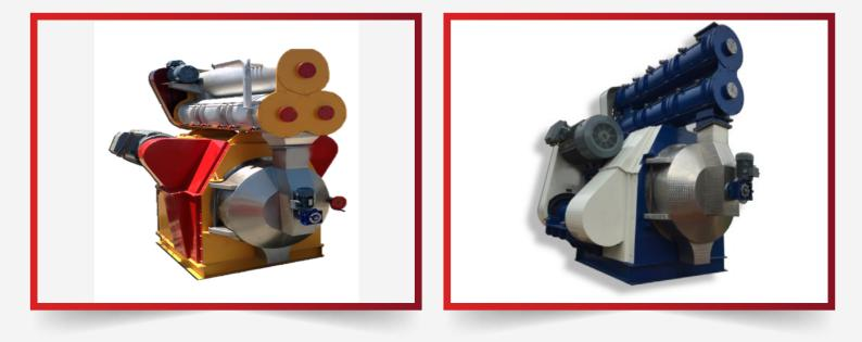
These are machines where the raw material of the pelleting process is transformed into a product. The product to be pelleted is fed to the pellet press after drying and grinding.
