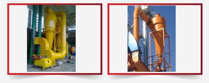
Dust cyclones are dust filters that allow the air entering into it to fall to the cone under it by following the helical path. Through to the air locks on the lower cone of the cyclones, it allows the dust in the cyclone to be collected from the bottom of the cyclone without absorbing air from the outside.
