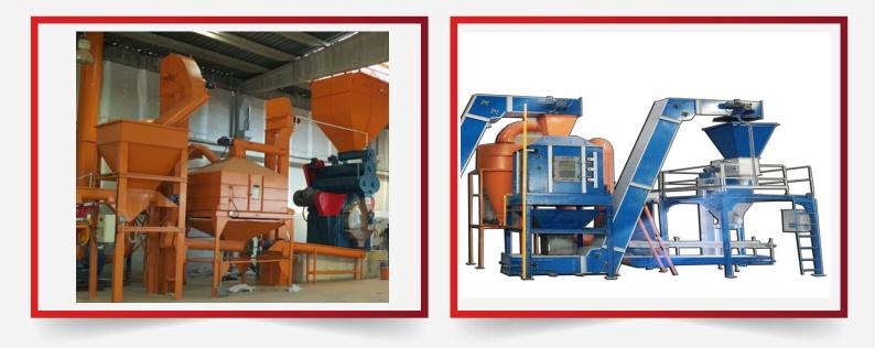
The pellet product coming out of the pellet press is affected by the ambient humidity and is a machine that works with reverse air flow that prevents it from becoming sludge. If the pellet is allowed to cool by itself, sludge, transverse and longitudinal cracks occur and this degrades the quality of the pellet. It causes pollination in the pellet.
